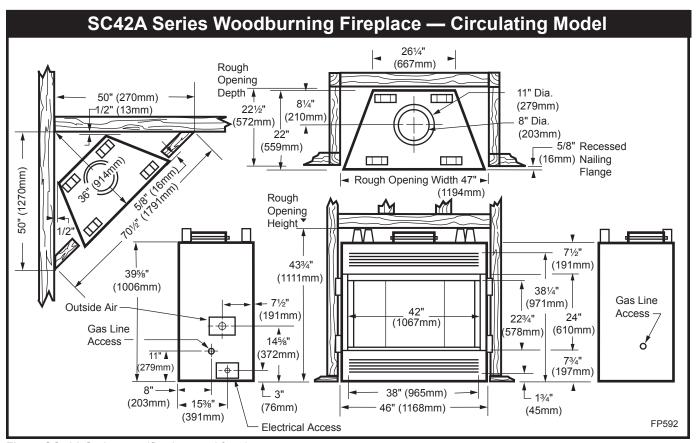
Fig. 4 SC42A Series specifications and framing.
